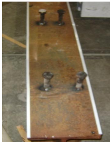
Figure 21: Girder with HDPE Strips
