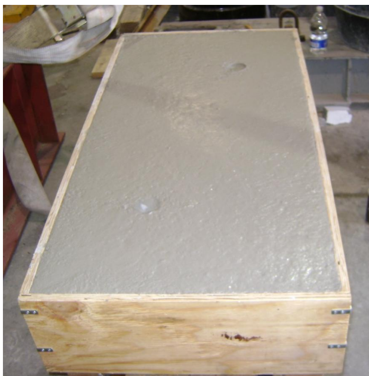
Figure 27: Specimen after Concrete Placement
