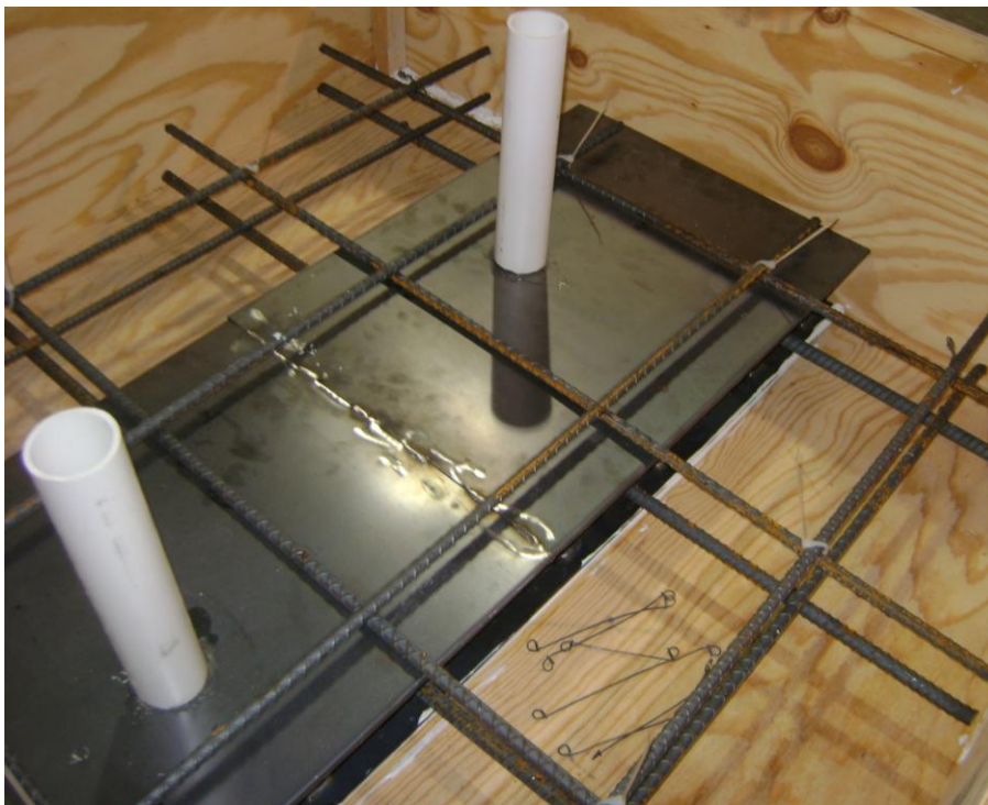
Figure 34: Specimen with Reinforcement
