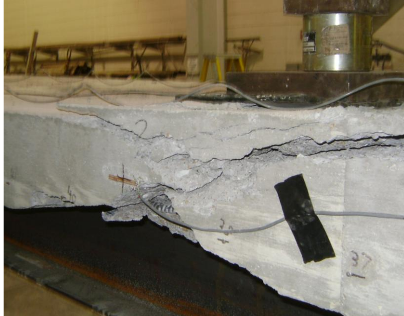
Figure 85: Compression Failure at Mid-span
