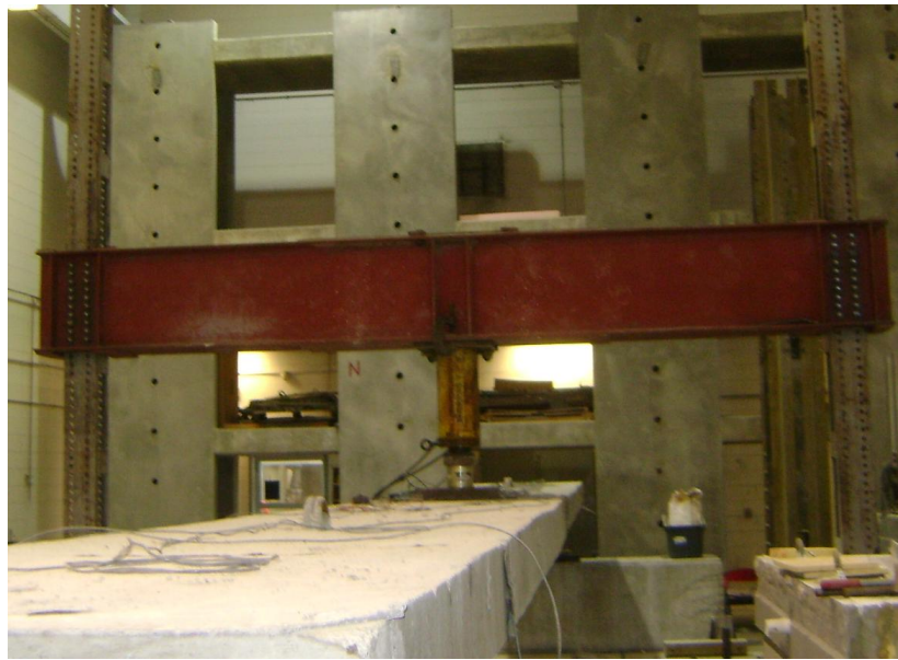
Figure 83: Flexure Test Setup
