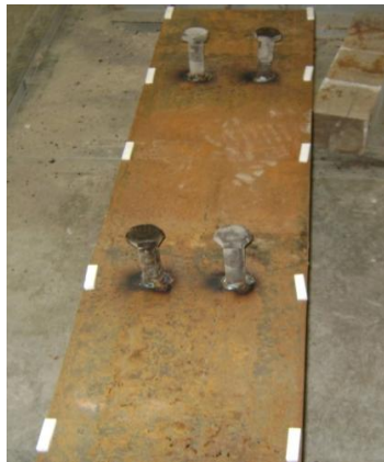
Figure 20: Girder with Teflon Strips
