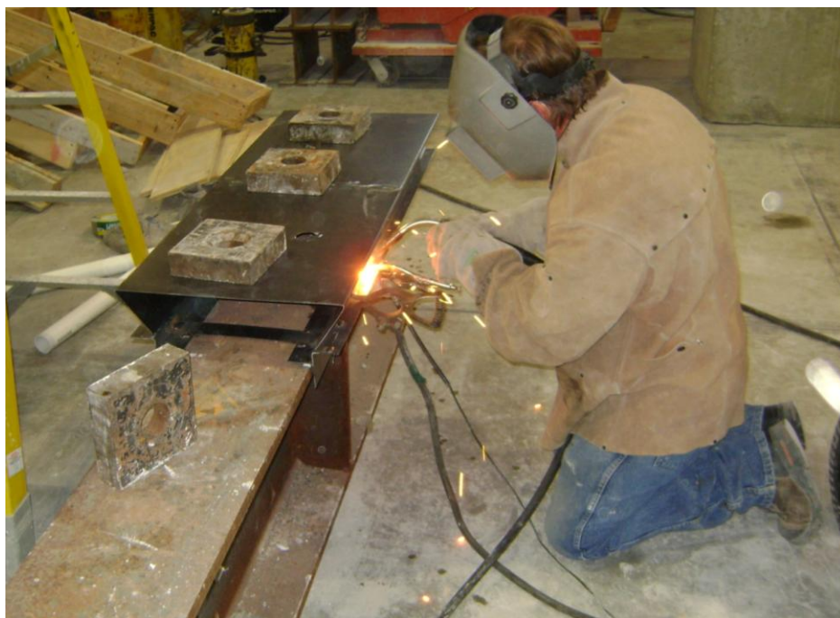
Figure 32: Welding of Specimen
