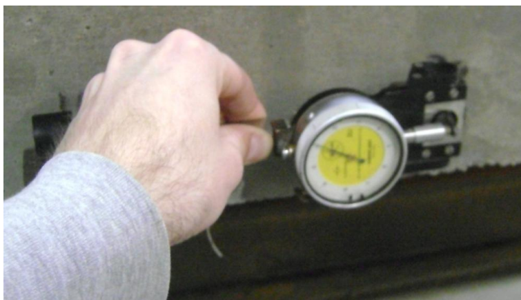
Figure 68: Instrument for Measuring Change in Strain of Demec Gauges
